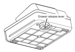
In case of power failure or the machine is in malfunction, the cash drawer does not open automatically. Even in these cases, you can open the cash drawer by pulling drawer release lever (see below).
