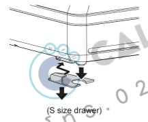
Drawer hook prevents the cash register from falling caused by weight of coins.
